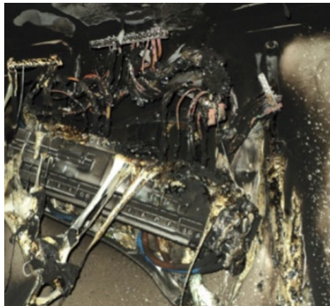
Fig 1. Consumer unit with plastic enclosure after a fire caused by a loose neutral termination
