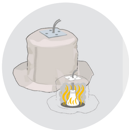
Typical fire hood for a downlighter
