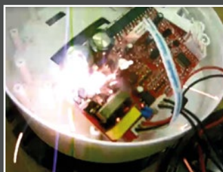
△ Component failure resulting from a short-circuit.
