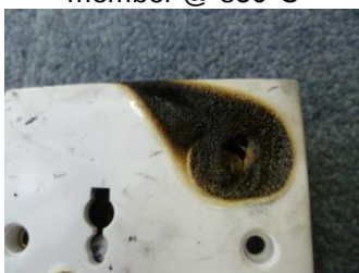
Sample 1 switch actuating member @ 850°C
