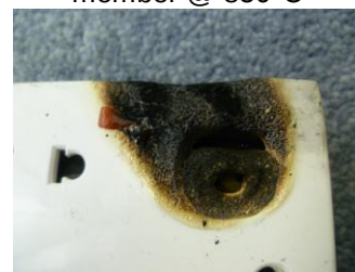
Sample 3 switch actuating member @ 850°C
