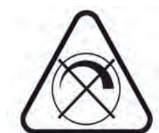
Fig 16. Symbol that lamp is not suitable for use with a dimmer switch.
