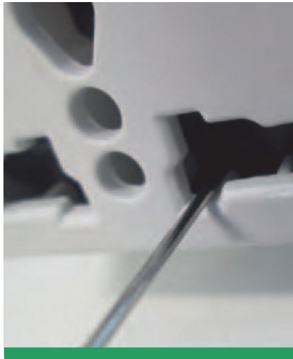
Fig 3. Access to live parts
