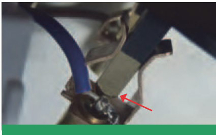
Fig 2. Soldered connections in the accessory prevented the test plug being fully inserted
